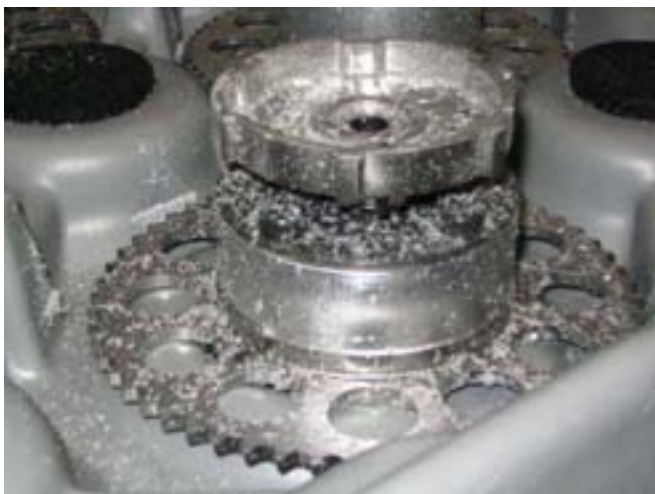
Standard HPDE produces plastic shavings
